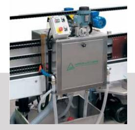
The washing machine applied to the **edging machines and bevelling machines** outlet conveyor allows the complete cleaning and drying of the processed edges of the glass sheets.
